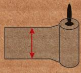
**Pre-Stretch Film** Pre-stretch film should be held with just enough tension to make the edge stand up but not so tight as to cause neck down. **Blown or Cast Film** When applied with the optimum level of stretch the film will neck down.
