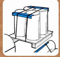
Cornerboards provide effective palletising and packaging for cylindrical products such as paper rolls, coils, drums etc.
