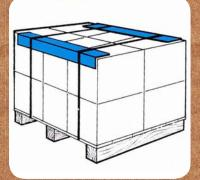
Cornerboards can be used with shrink or stretch film to reduce damage and improve presentation of merchandise such as eggs and wine.
