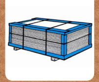
Cornerboards protect panel products from edge corner damage and shifting of the load.
