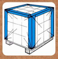
Cornerboards unitize light and easily damaged cartoned products, eg potato chips, biscuits etc.
