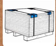
Cornerboards increase the effectiveness of 'strapping and eliminate strap damage.
